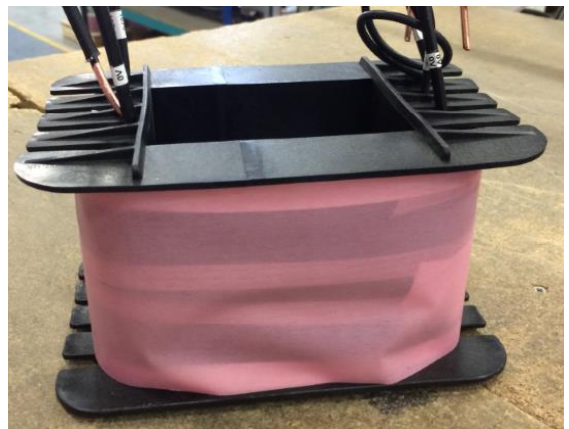
Bobbin wound EI3.00/ 9A x 5" coil ready for insertion of lamination
