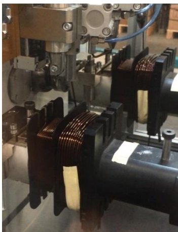
Two spindle, simultaneous automatic winding of EI212 plastic, 3 flange bobbins
